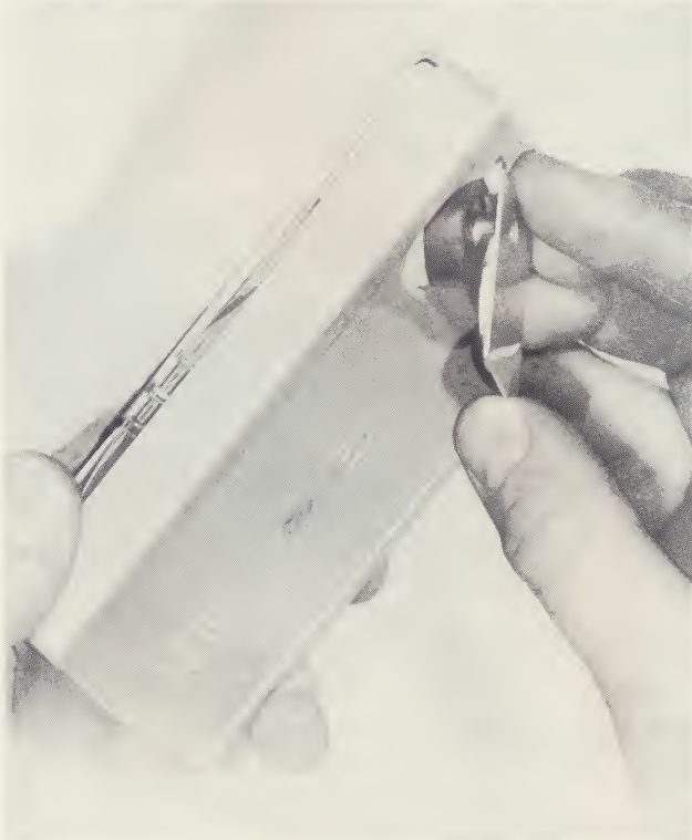
Pinch roller being inserted into magnetic tape cartridge.
